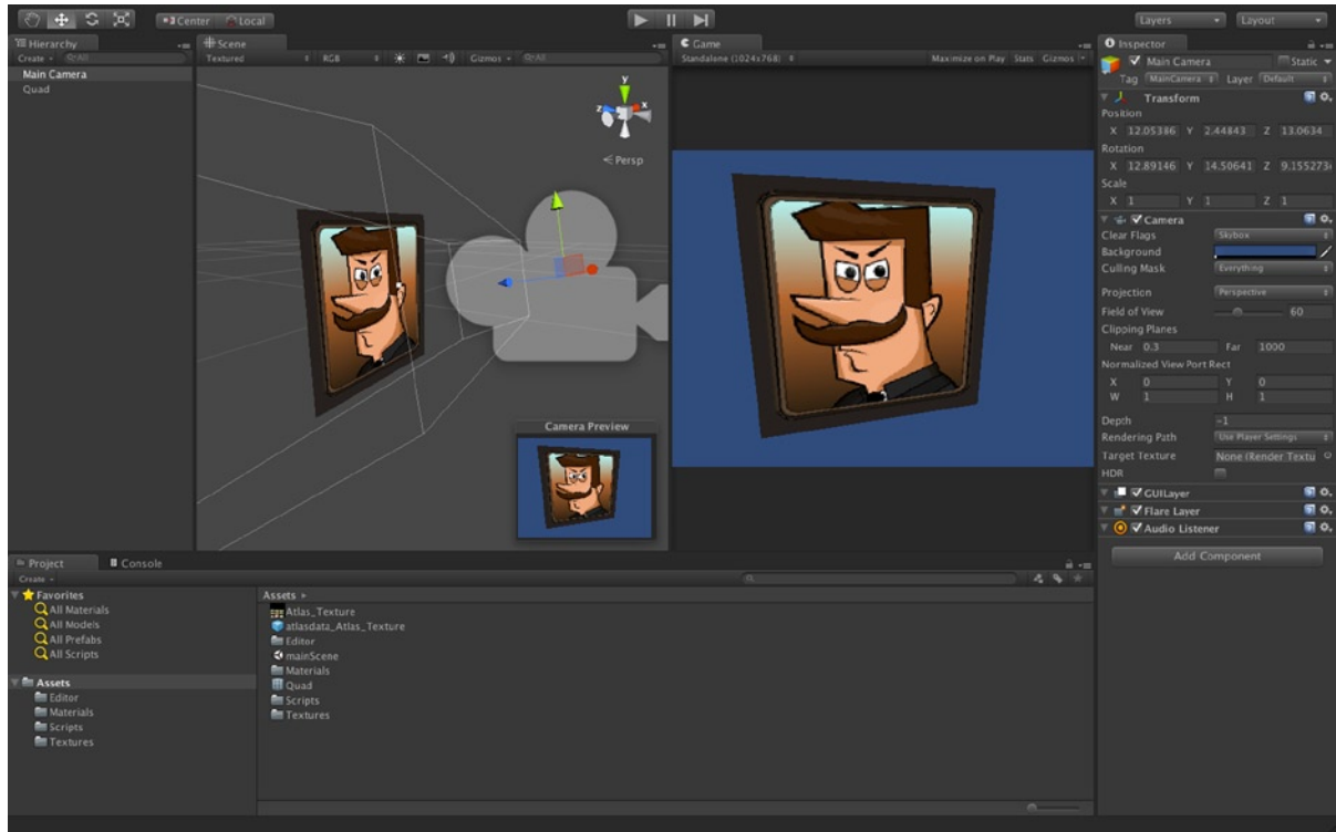
Figure 8-1. Textured Quad in perspective view. Texture is not pixel-perfect and there is no obvious relationship between world space (in Unity Units) and screen space (in Pixels)
