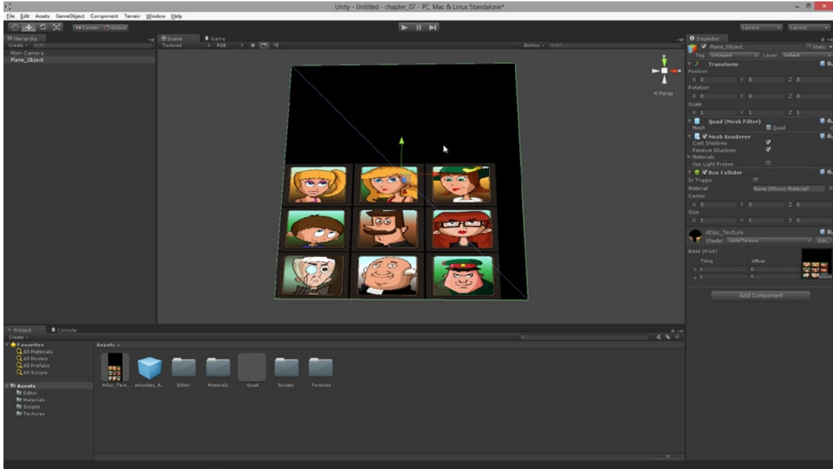
Figure 7-1. By default, textured quads are generated with UV mapping to show a complete texture, from the top-left corner to the bottom-right corner. This does not meet the needs of Atlas Textures. To fix this, we'll need to edit the mesh UV mapping
