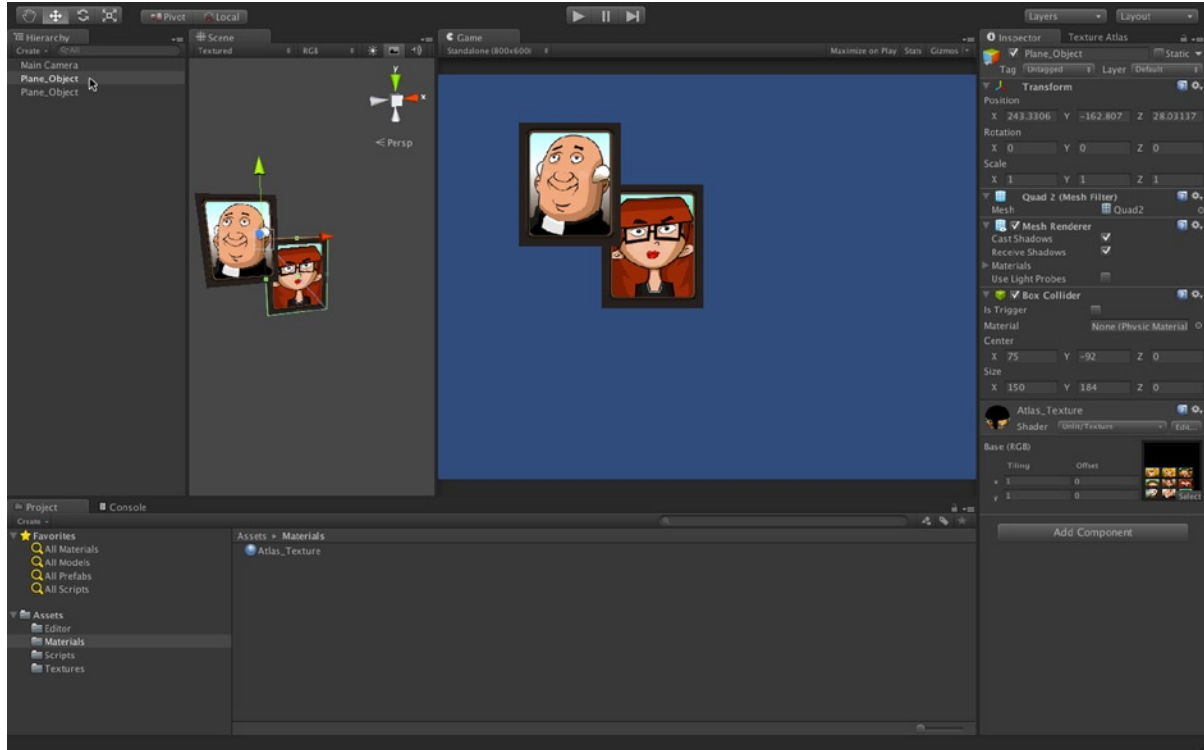
Figure 8-16. Control game object Z-Order (Depth) using the Z (Depth) value of an object's Transform component. The woman sprite is offset further back on the Z-axis and appears behind the male character sprite in the game Viewport
